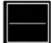
If THE APU is OPERATING PRESSING THE [ ] will shutdown THE APU IMMEDIATEly. This is STRONGLy discouraged BECAUSE THE cool-down PERIOD is BYPASSED AND COMPONENT DAMAGE is likely
