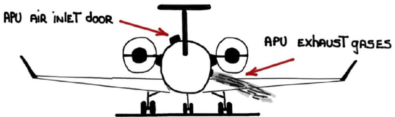
To PREVENT damage to the engine cowls WHEN OPENED during ground maintenance THE APU STARTER is inhibited
