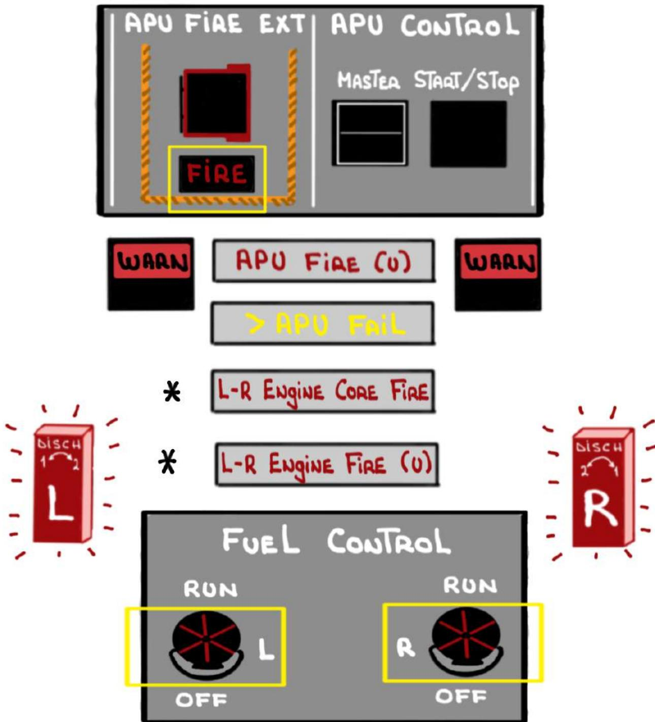
If on the ground a fire bell (located in the nose wheel well) will sound
