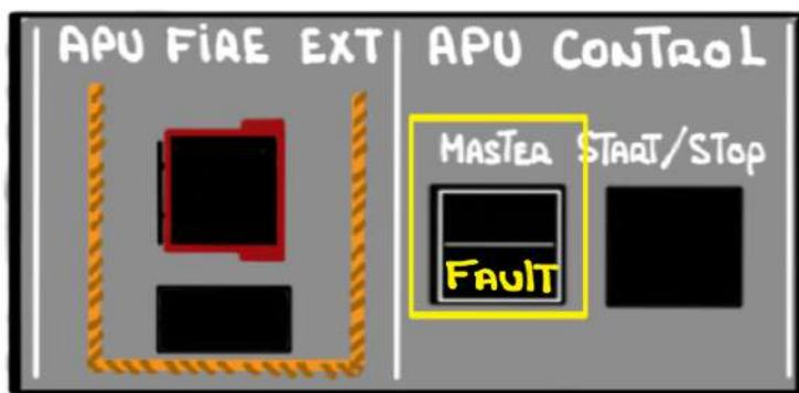
THE MASTER switch CAN BE CYCLED OFF AND ON IN AN ATTEMPT TO CLEAR THE FAULT
