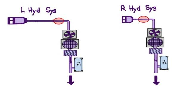
· ELECTRO-Hydraulic Servo AcTUATOR
