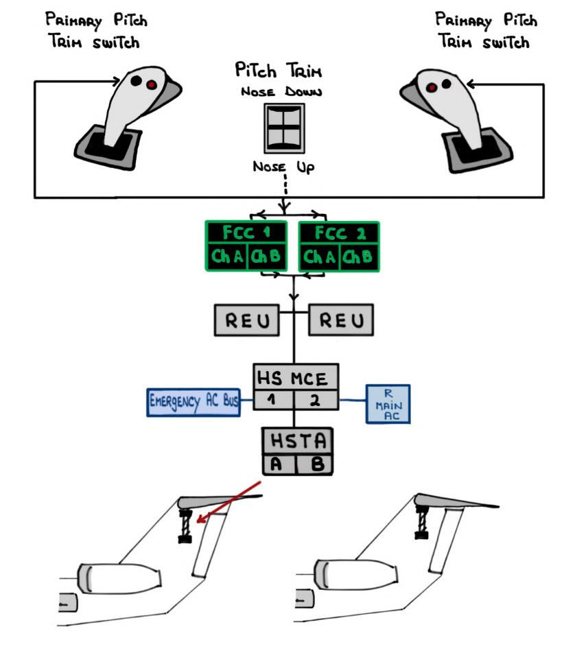
In the event of loss of communication from the FCCs The sidestick pitch trim switches won't be available. The pedestal switch bypasses the FCCs and signals the HS MCE. The stab moves at a constant rate
