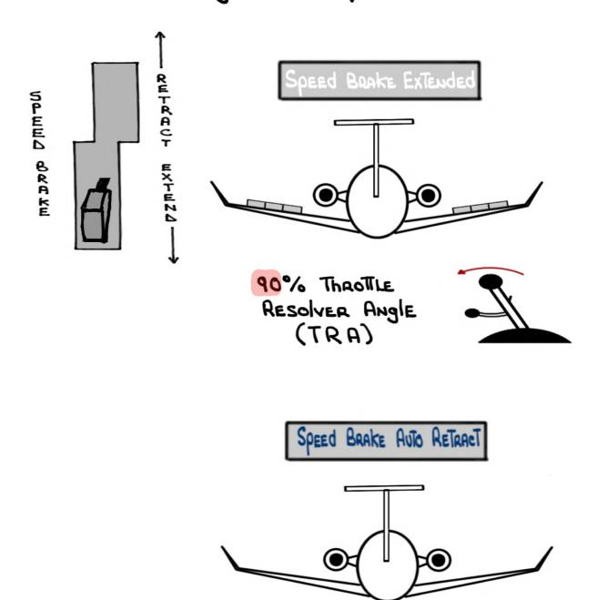
Speed brakes <u>retarct</u> but speed brake handle does not
