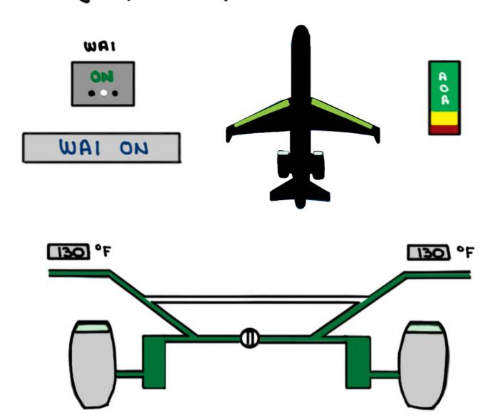
Wing Temperature MUST be > 100°F and Aircraft
