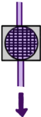
Filter Manifold: To filter hydraulic fluid AND CONTROL direction of flow
